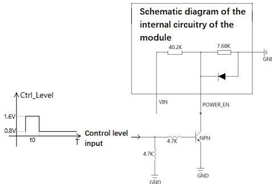
**POWER\_EN** foot and **GND** access module, MCU connected to the microcontroller, the motherboard power-up so that the control level output high, transistor conduction, **POWER\_EN** foot is low, the module does not start; power supply stabilization so that the control level has been at a low level, the transistor cutoff, the **POWER\_EN** foot is a high level, the module is normal operation.
