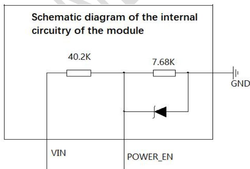
The control module delayed start circuit reference design has the following two options:
